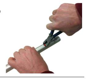
2. Removing the red spring from the tube is best done using a medium/small screw driver. Push it towards the tube hole and fiddle until you can remove it completely.
